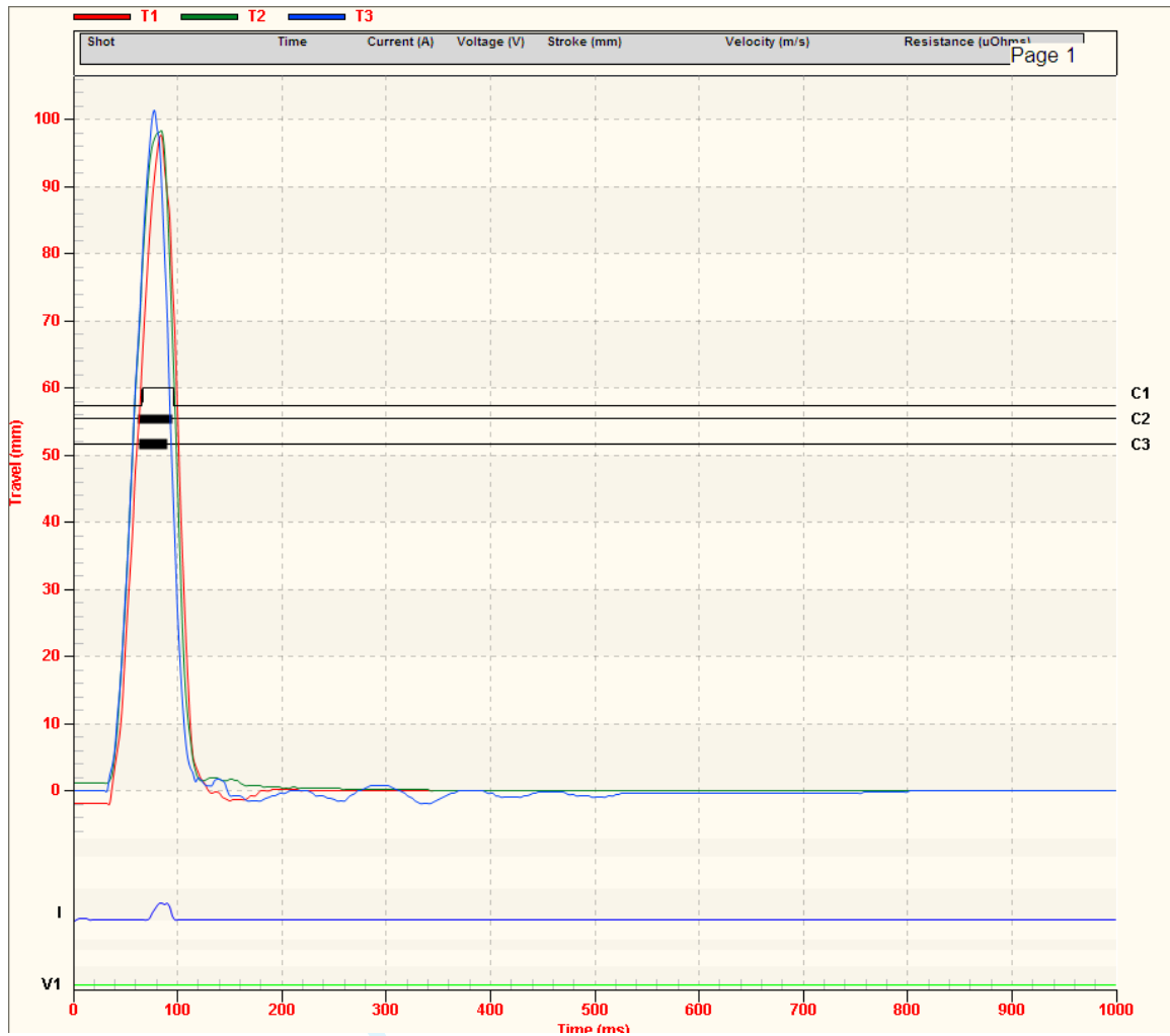
Figure 3. Graph Showing Contact Channels in Analog (C1) and Digital Format (C2 and C3)
