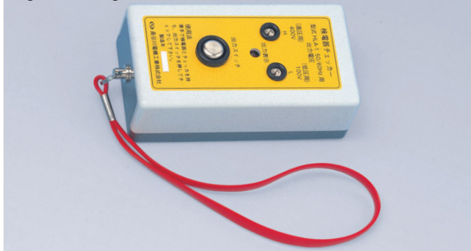
Figure 6: Voltage detector checker
