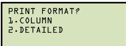
Press the **[1]** key (*COLUMN*) to print a columnar report (see Figure 16) or press the **[2]** key (*DETAILED*) to print a detailed report (see Figure 17).
