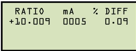
The polarity is displayed as either a plus sign (+) for “in-phase” or a minus sign (-) for “out-of-phase”. The value listed under “% DIFF” is the percentage error.
