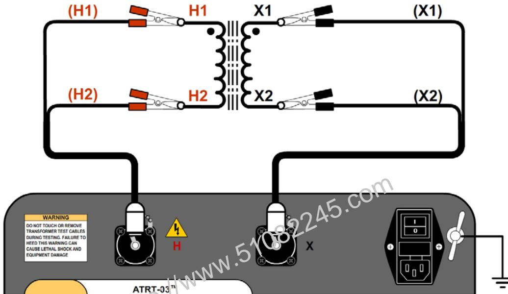
Figure 7. Typical Connections to a Single Phase Transformer
