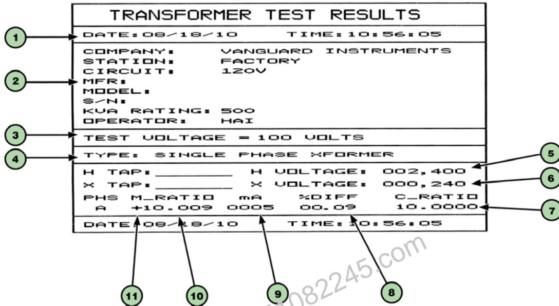
Figure 16. Single Phase Test Results Printout - Column Format
